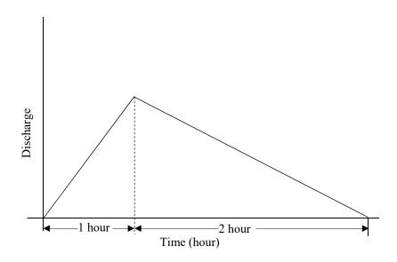
The peak discharge (in m<sup>3</sup>/s, *rounded off to one decimal place*) of the above unit hydrograph is \_\_\_\_\_
