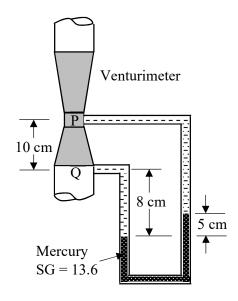
Taking specific weight of water as 9810 N/m<sup>3</sup>, the pressure difference (in Pa, *rounded off to one decimal place*) between point Q and P is \_\_\_\_\_.
