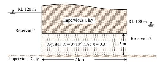
If the Reservoir 1 is contaminated by a pollutant then the time (in days, *rounded off* to one decimal place) taken by the pollutant to reach to the Reservoir 2 under advection will be \_\_\_\_\_\_.
